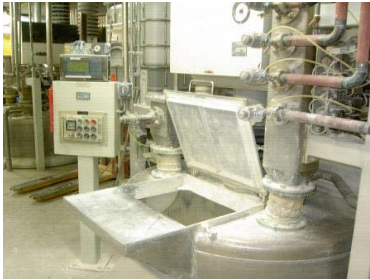
Figure 6: Dissolver directly connected with storage tanks
