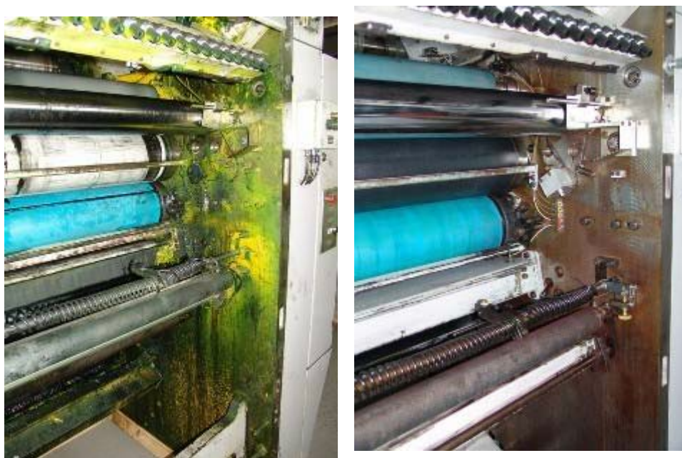
Figure 5: Printing machine before and after cleaning with dry ice
