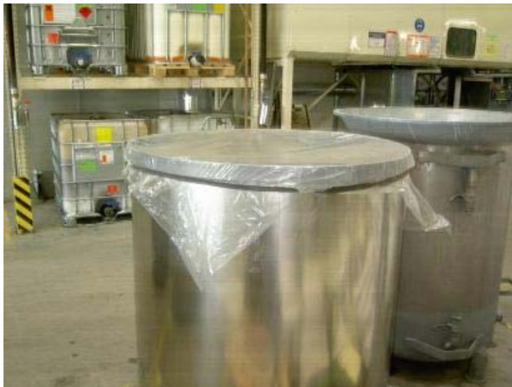
Figure 7: Interim storage of containers covered with antistatic foil
