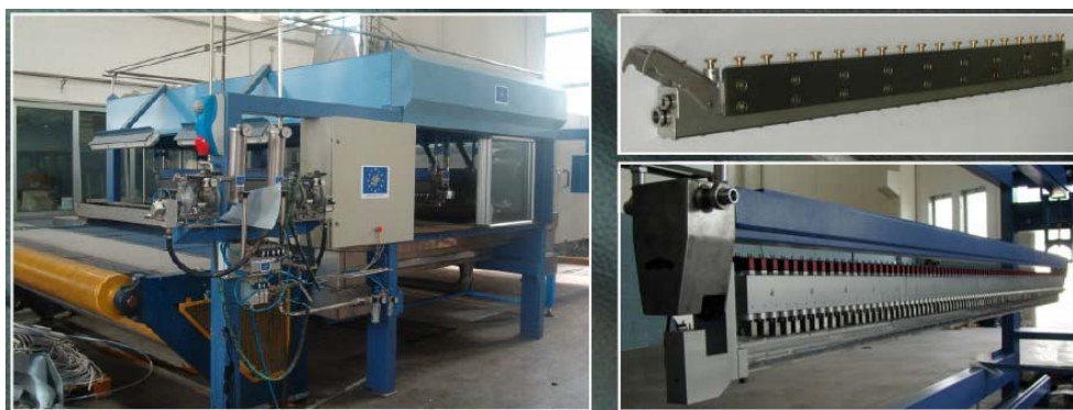
Figure 3: Conveyor belt spraying booth and oscillating bars with spray gun nozzles
