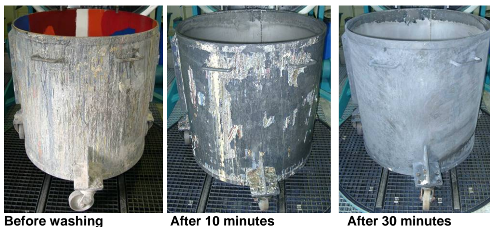
Figure 5: Automatic water based alkaline washing of vessels
